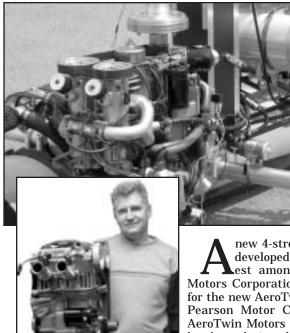
At 65 horsepower and "less than 80 pounds ready to run," the new AeroTwin 4-stroke aircraft engine, designed and manufactured in New Zealand, is expected to "meet the needs of several markets for a lightweight yet powerful engine," says worldwide distributor AeroTwin Motors. The first application should be the AirScooter II "Part 103 recreational vehicle" - a helicopter.
